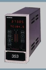
The Model 353 Process Automation Controller (PAC) is designed for a broad range of process applications. It can serve as an advanced singleloop controller or as a multiloop controller with complete control functions, including indication, control, logic, or sequencing for a small unit process.
