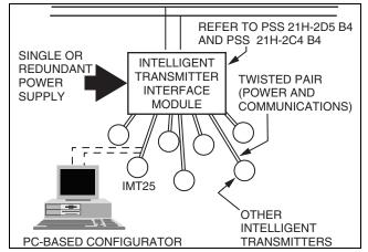
Figure 5. FoxCom Only Digital Output Functional Block Diagram
