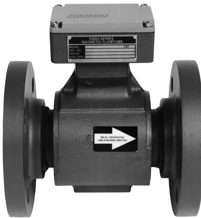
These pfa, ptfe, and polyurethane-lined compact, flanged magnetic flowtubes, together with an IMT25 or IMT25L Magnetic Flow Transmitter combine to form an easy-to-use versatile, dc pulsed Magnetic Flowmeter. The flowmeter measures electrically conductive liquids and produces a measurement signal directly proportional to volumetric flow rate. As symbolized by the CE logo marking on the product, the flowtube conforms to the applicable European Union directives.
